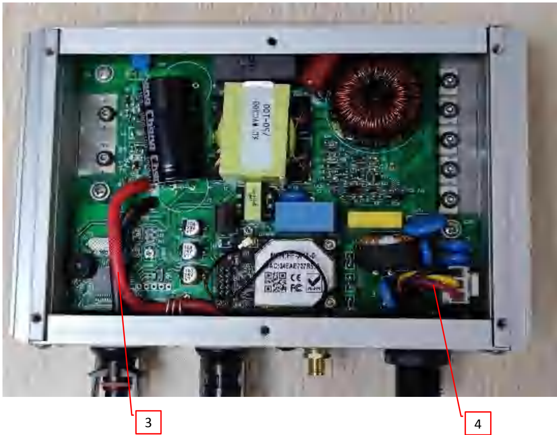
Photo 5 - Internal view of the unit (before Pouring sealant)
